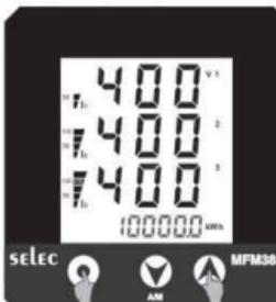
Display shows line to line voltage (V<sub>LL</sub>)
