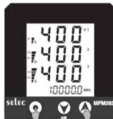
Display shows Line to Line Voltage (V.L.) & Energy.
