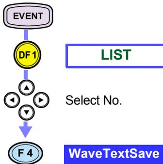
To save multiple event waveforms, select a number (No.) and repeat the process.
