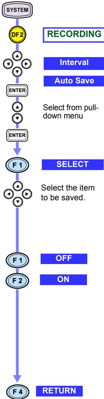
Measured data files are saved to the PC card with the internal memory automatically.
