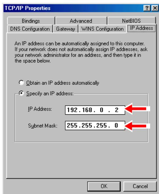
3. Confirm the IP address and subnet mask for the computer you are using.
