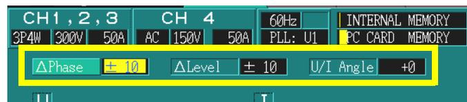
**ΔPhase** Tolerance level of each phase in the phase range
