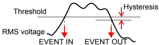
**Swell** is detected when the RMS voltage RMS exceeds the threshold in the positive direction.
