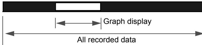
The waveform display range (white belt) on the scroll bar indicates what interval of recorded data is displayed on the screen.
