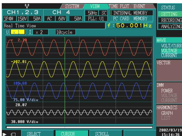
Displays voltage waveforms for channels, depending on how they are connected.
