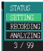
When the repeated recording function is set, the number of repeated recording operations currently set will be indicated.
