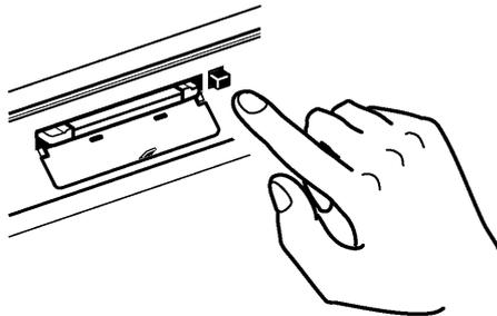
Press the eject button and pull out the PC card.
