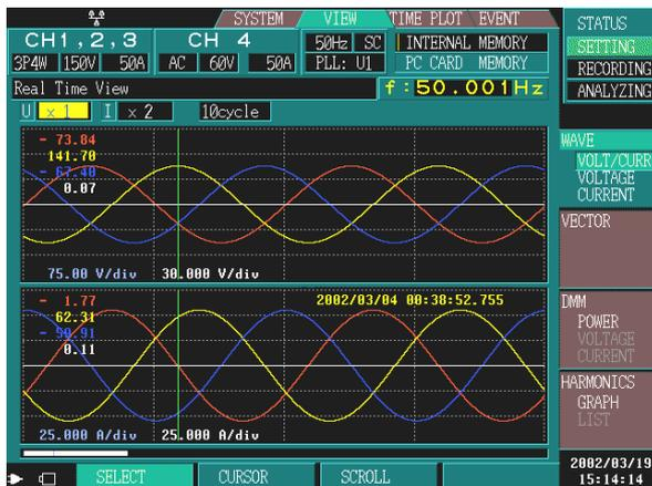
Displays voltage and current waveforms for channels, depending on how they are connected.
