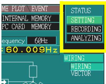
Screen operations are limited according to the internal operation status.
