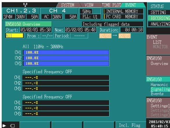
Displays detailed judgment results for signaling voltage, in accordance with the EN50160.
