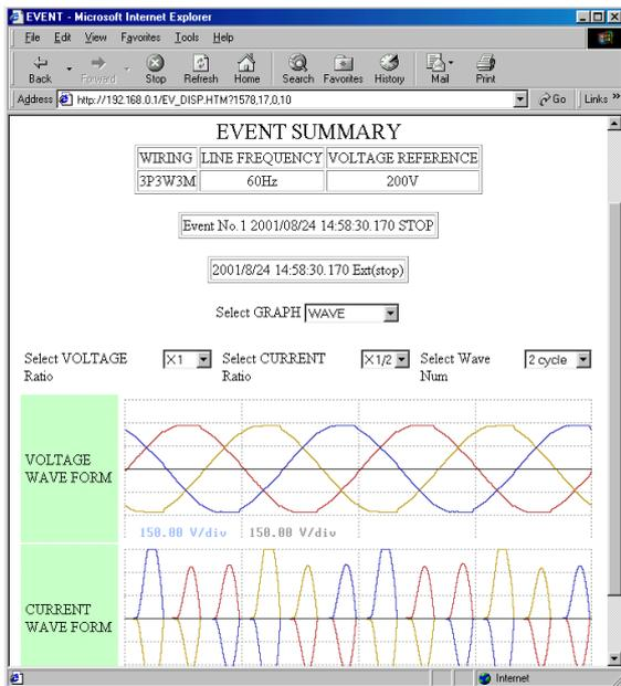
You can select the voltage, current, and waveform scales.
