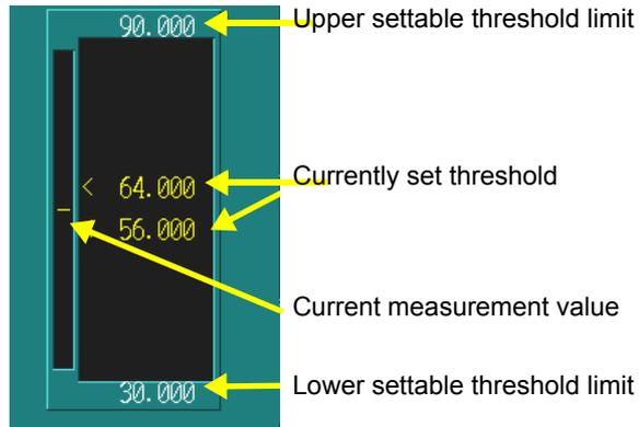
Thresholds can be set while viewing the current measurement values.
