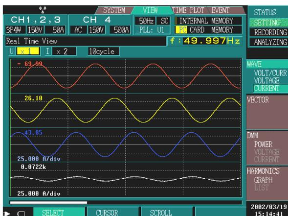
Displays current waveforms for channels, depending on how they are connected.
