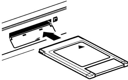
Open the cover and insert the PC Card with the arrow facing up and in the direction of the PC card slot, as far as it will go.
