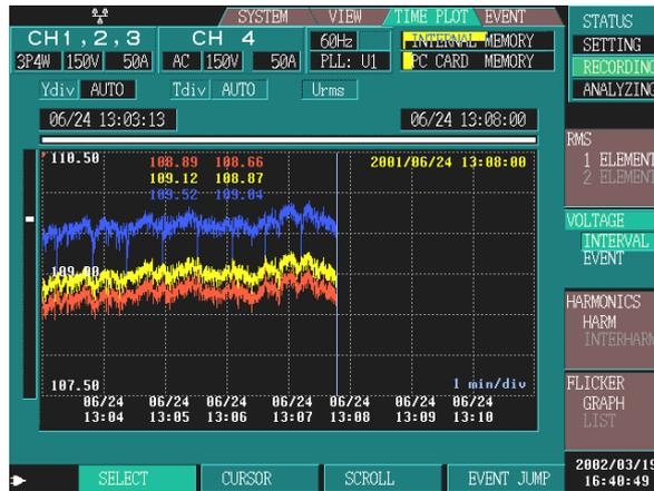
Displays a voltage fluctuation graph used to calculate the swell, dip, and instantaneous interruption.
