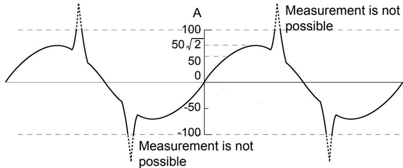
A measurement device with a small crest factor
