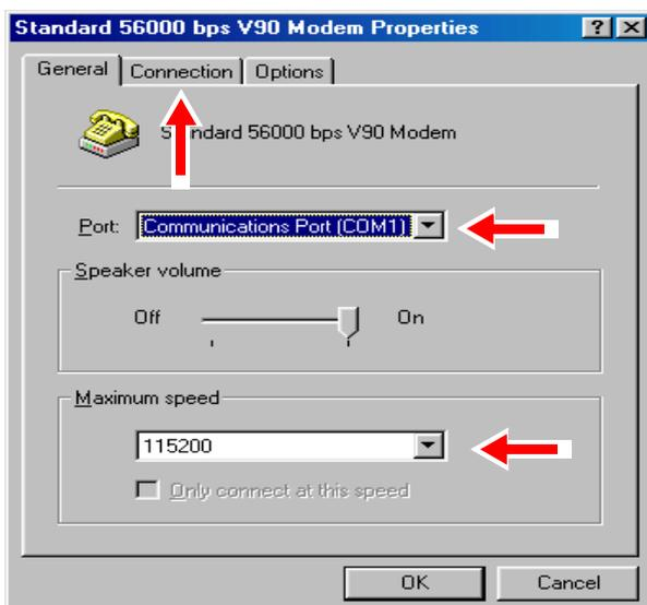
4. Check that the communications port is the same port that the modem is connected to.
