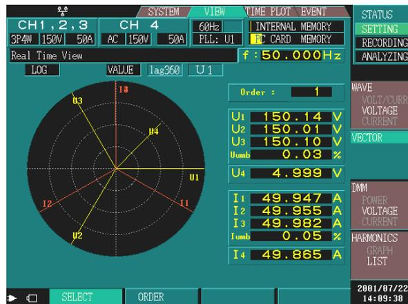
Displays voltage and current vectors for channels, depending on how they are connected.
