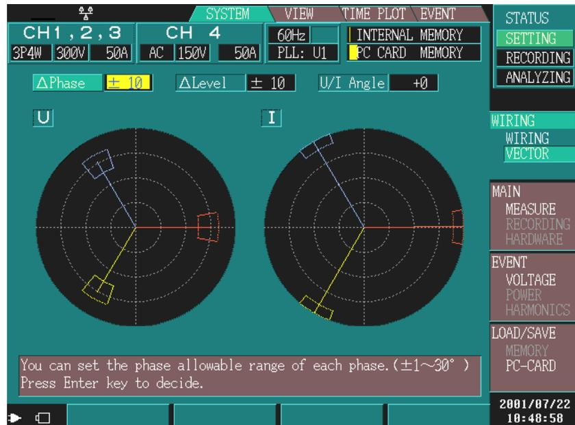
You can check the voltage and current vectors of each connection method.
