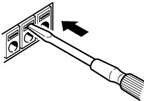
1. Press down on the terminal button using a tool, such as a flat head screwdriver.
