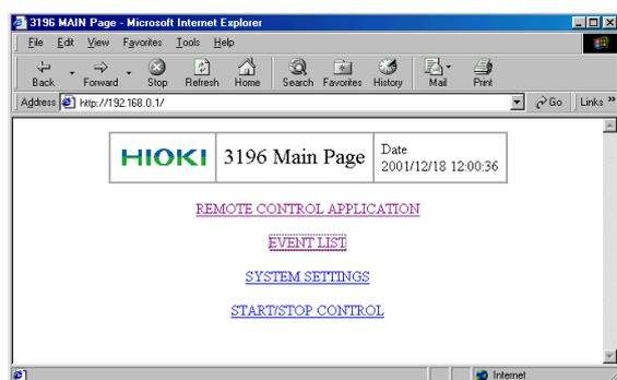
Start up Internet Explorer, and enter the IP address that you set for the instrument (example: <http://192.168.0.1/>) in the address column, then press the Enter key.
