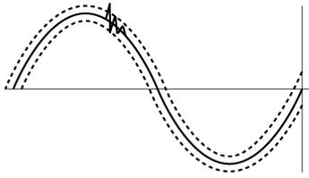
Reference waveforms are formed above and below the voltage waveform with an interval of 200 ms and with an offset equivalent to the threshold value, then detection is performed by comparing the measured waveform with these reference values.
