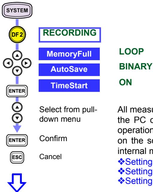
All measured data collected by repeated recording is stored on the PC card, but previous data is cleared in each recording operation and not retained in internal memory (data displayed on the screen). Therefore, only the latest data is retained in internal memory at any given time.
