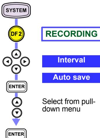
Measured data files are automatically saved to the PC card with the internal memory.
