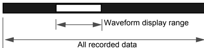
The waveform display range (white belt) on the scroll bar indicates what interval of recorded data is displayed on the screen.
