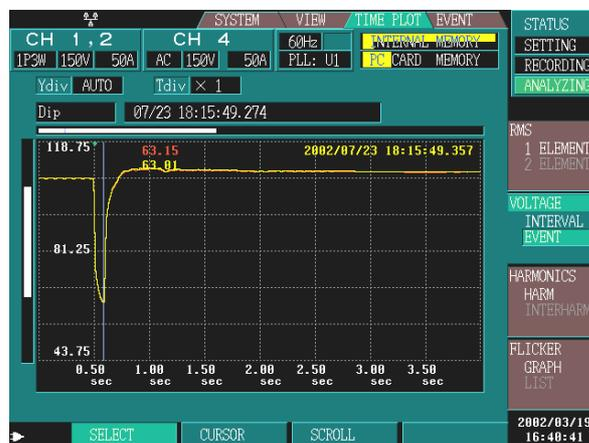
Displays the voltage fluctuation graph for a voltage swell, dip, or instantaneous interruption event.
