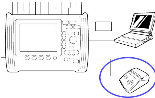
Using the device's RS-232C interface, you can create hard copies of the 3196 screen with the 9670 PRINTER.
