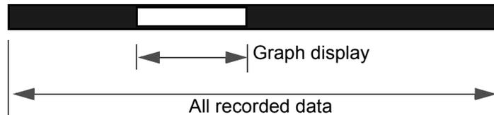
The graph display range (white belt) on the scroll bar indicates what interval of recorded data is displayed on the screen.
