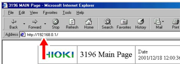
4. Start up Internet Explorer, and enter the IP address that you set for the instrument (such as http://192.168.0.1/) in the address column, then press the Enter key.
