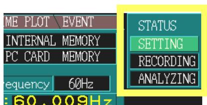
One of **[SETTING]**, **[RECORDING]**(**[WAITING]** until preset time to start measuring), or **[ANALYZING]** is displayed to indicate the internal status of the instrument. The internal status is changed by pressing **START/STOP** to start/stop recording.
