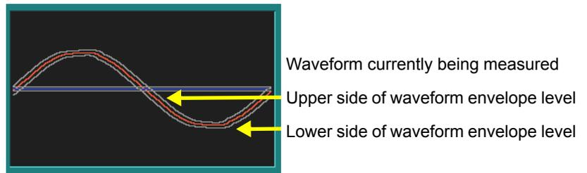
When the measured waveform exceeds the waveform envelope level, a voltage waveform comparison event is generated.
