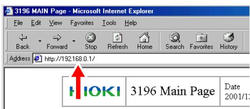
Start up Internet Explorer, and enter the IP address that you set for the instrument (such as `http://192.168.0.1`) in the address column, then press the Enter key.
