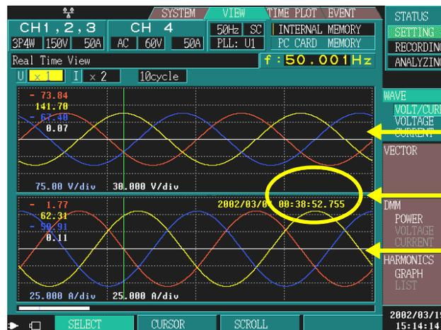
Superimposes and displays 4 channels of the voltage waveform.
