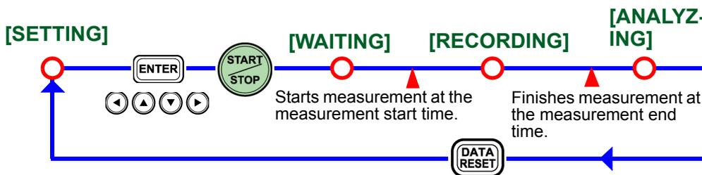
If the preset measurement start time has already passed, measurement starts immediately.
