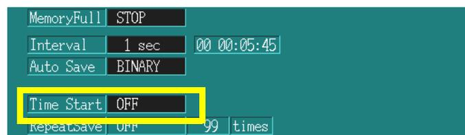
**OFF** Measurement starts or stops when you press the START/STOP key.
