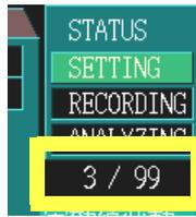
When the repeated recording function is set, the number of repeated recording operations currently set will be indicated.
