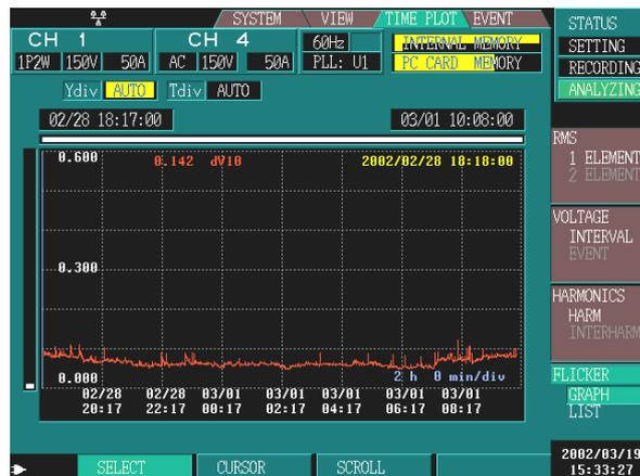
Displays a fluctuation graph for  $\Delta V_{10}$  flicker.
