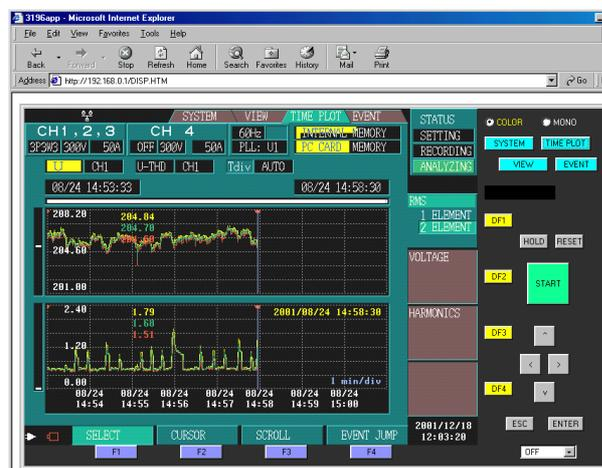
The screen displayed on the Internet browser is the same as the screen displayed on the instrument with the same key placement as the front panel.
