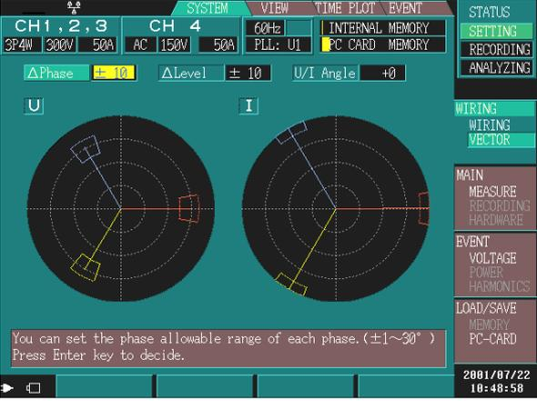
The screenshot shows two vector diagrams, one for voltage (U) and one for current (I). Below the diagrams is a text box:
