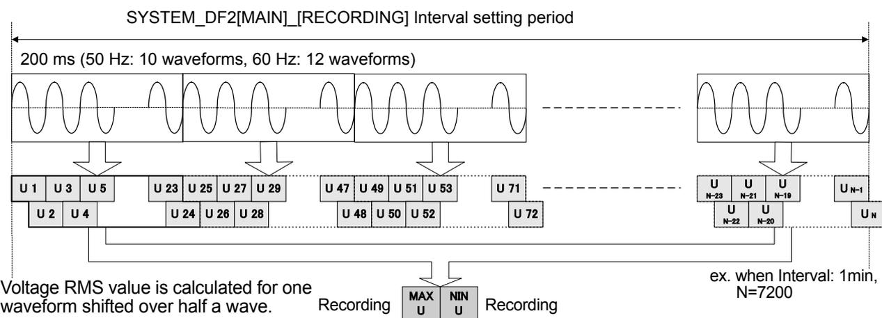
Voltage RMS value is calculated for one waveform shifted over half a wave.
