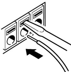
2. While the button is depressed, insert the wire into the electric wire connection hole.
