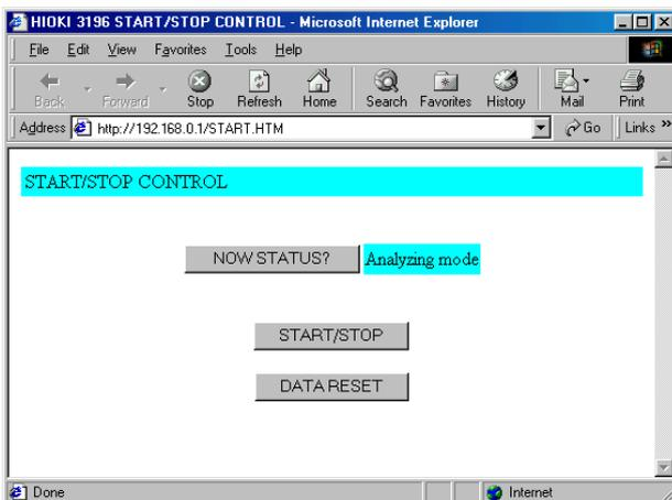
This screen allows you to start and stop measurement, and execute the data reset control for the instrument.
