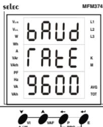
**Baud Rate****Default Setting:** 9600.**Range:** 300, 600, 1200, 2400, 4800, 9600 & 19200**Note:** The baud rate could be one of the seven, 300, 600, 1200, 2400, 4800, 9600 & 19200
