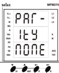
**Parity****Default Setting:** None**Range:** None, Even, Odd**Note:** For asynchronous communication, user can select any one of three None, Even, Odd
