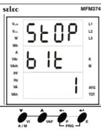
**Stop Bit****Default Setting:** 1**Range:** 1 or 2**Note:** For asynchronous communication, user can select any one from '1 or 2'
