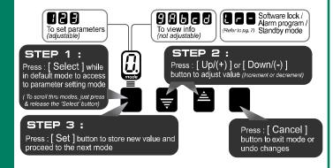
All modes exit automatically if left untouched for more than 20 seconds. (For fast increment or decrement, press and hold the UP or Down button)
