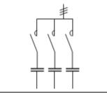
The in-rush current of such high magnitudes is undesirable and it is likely to weld main poles of any standard contactor.
